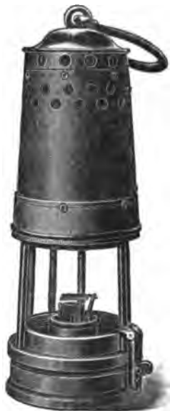
FIG. 76. Miner's lamp fitted with the Cunynghame-Cadman device.
